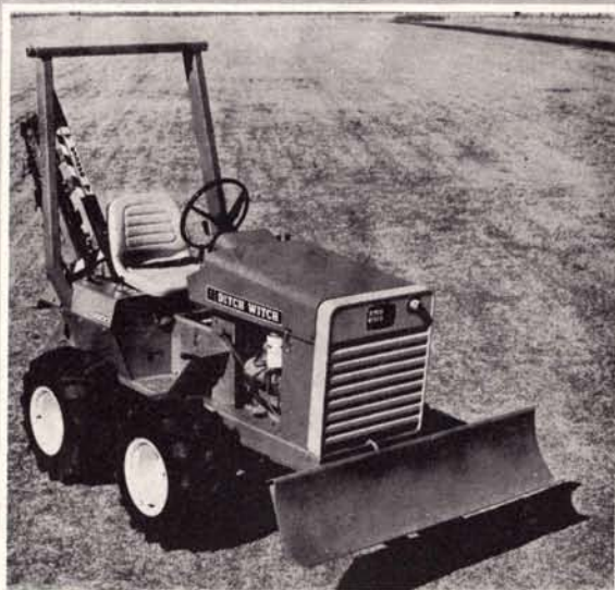
The Ditch Witch Model 2200 with optional roll over protective structure and flotation tyres.
